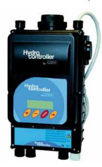
Professional water-through VFD (Variable Frequency Drive) for residential and industrial applications (in line type, cooled by water). It controls the start&stop of the electric pump, adjusts the motor speed according to the actual water demand and keeps the desired pressure constant. The Hydrocontroller is suitable for booster sets with a maximum of 8 pumps in serial connection. It assures high energy saving and important advantages in terms of comfort, performance and durability of the system.
