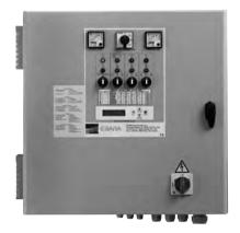
Control panels with inverter SP series modulate the operation of electro pumps responding to the pressure trasducer control (measured by flow rate or other external signal 4-20 mA passive) adjusting the speed of the electric pumps to maintain constant the system demand.
