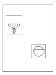
Control panels for fire-fighting units in compliance with EN 12845 for compensation electric pumps.
