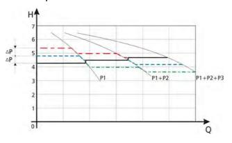
To do this, enter the amount of pressure drop you will allow before the next pump starts (=value of parameter ACTUAL VALUE DECREASE). The diagram shows the pressure drop and increase.
